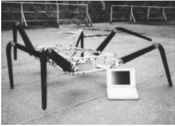
Figure 3: Photograph of the walking hexapod capable of walking on rough surfaces.
